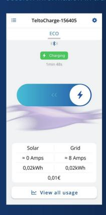
Charging station also supports communication with these energy meters for following data if Solar charging is ON:
